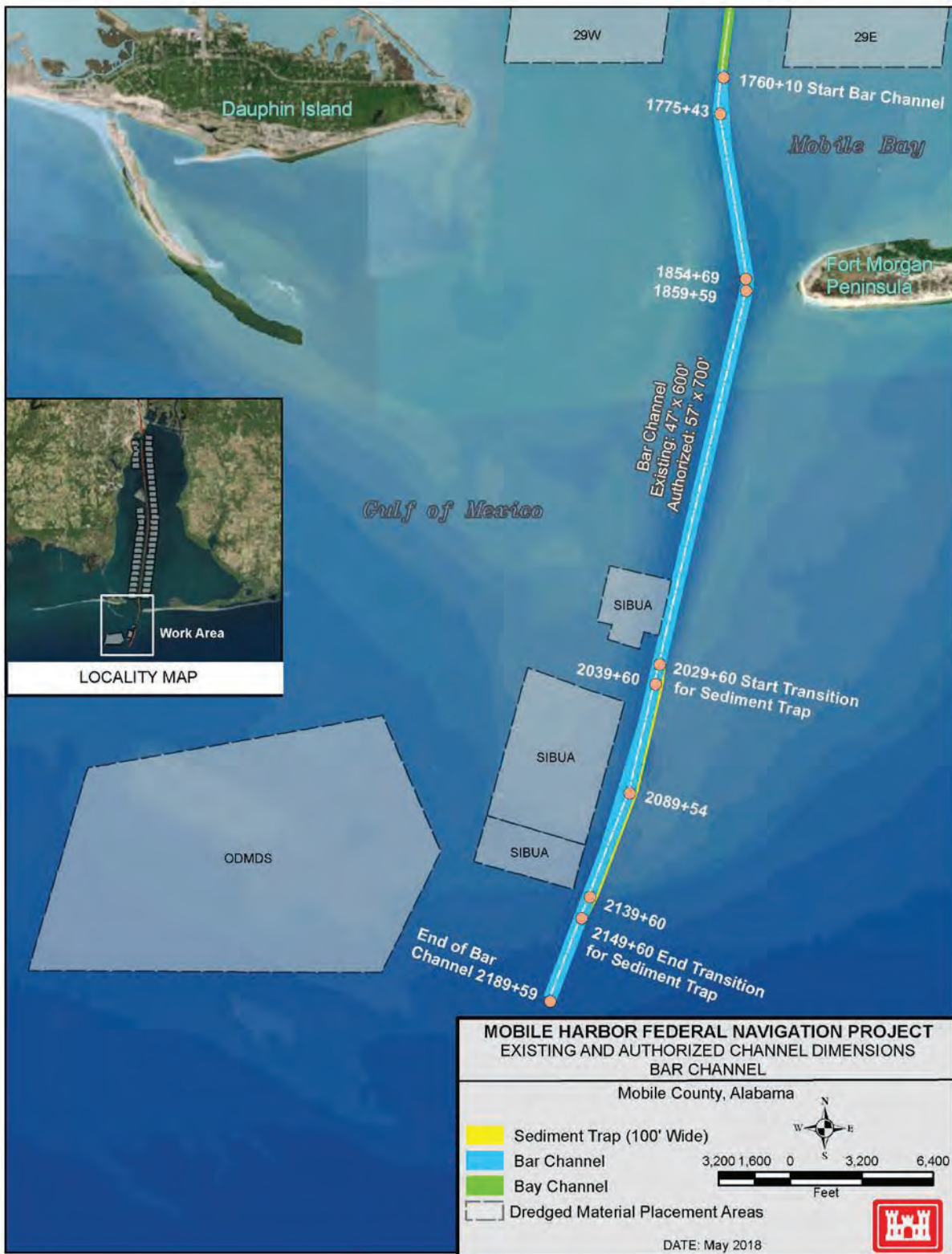
Figure 2-18. Bar Channel Alignment and Stationing
