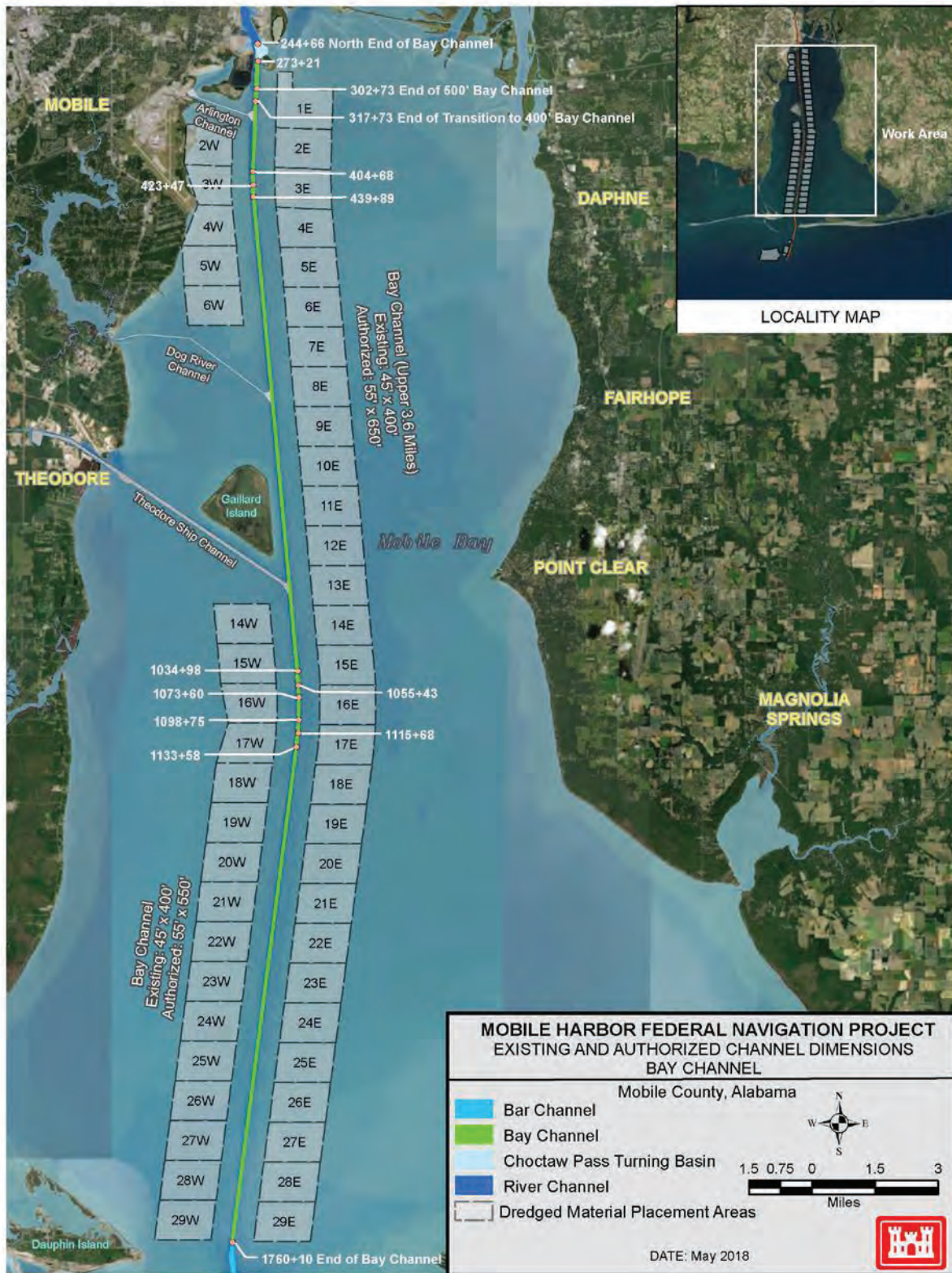
Figure 2-19. Bay Channel Alignment and Stationing
